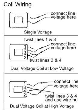
\* Refer to Figure 7 (page 5) for control circuit wiring.
