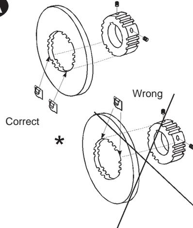
\* Stabilizer springs are for use on single disc units only. Position springs opposite set screw holes.
