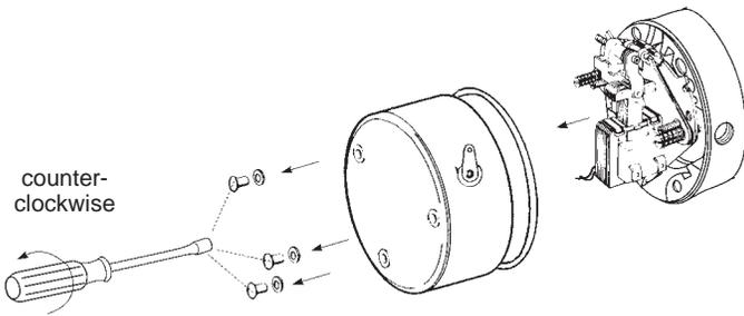
**5** Slide endplate over hub noting position of stabilizer springs, if used. (Refer to Friction Disc Replacement, View 4 and 4A.)
