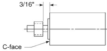
**3** Tighten set screws to motor shaft.
